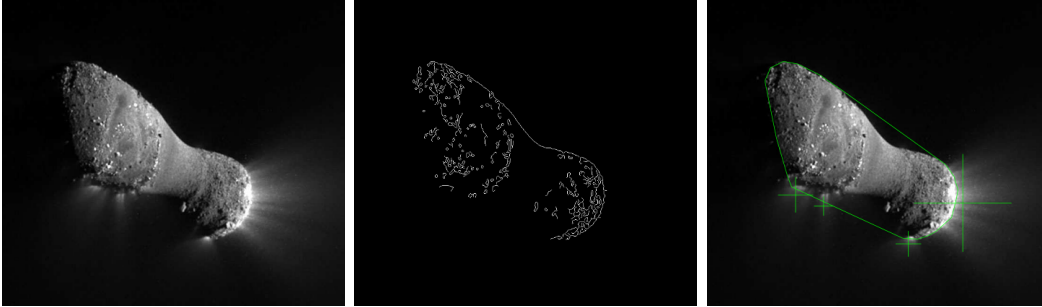
Figure 7: Left: Horizon models need not be ellipsoidal. Left: Nucleus of comet Hartley 2 as seen from the EPOXI flyby [4]. Center: Edge detection result. Right: Horizon identification using a convex hull, and subsequent detections of plume activity. Image credit: NASA/JPL-Caltech/UMD.
