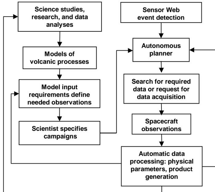
Figure 1. Layout of the Model-based Volcano Sensor Web (from Davies *et al.*, 2007). An alert of volcanic activity drives a request for data to be input into models of volcanic processes to gain a better understanding of the event taking place. Data are searched for; if not available, then assets are retasked to obtain the data. For example, detection of a volcanic plume leads to a request for data at short- and thermal-infrared wavelengths in order to estimate effusion rate.
