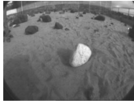
Figure 13. Sample image that was taken in response to a science alert indication identification of a rock with white albedo on the JPL FIDO rover.
